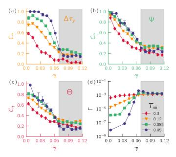
FIG. 6. Correlation decay from the as-cast glass and dissipation: Correlation decay  $C_{\gamma}$  at various degrees of stability (controlled by  $T_{\rm ini}$  in the POLY model) for the residual plastic strength  $\Delta \tau_{\gamma}$  (a), the vibrality  $\psi$  (b), and the steric bond order  $\Theta$  (c). Panel (d) shows the energy dissipation density  $\Gamma$  as a function of the strain  $\gamma$  for the same preparation protocols.
