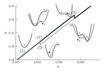
FIG. 5. Anelastic events in stable glasses: Example of an anelastic (reversible) plastic event in a stable glass (arrows indicate the loading direction). Rightmost sketches show the evolution of the potential energy landscape along the hysteresis.
