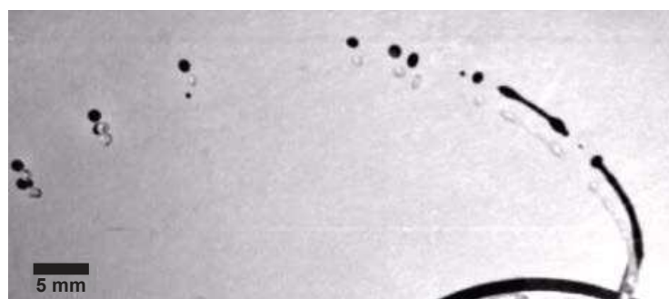
Figure 3.14: Image of the destabilization of a stretched ligament obtained with our experimental set-up. The liquid and its shadow are visible.
