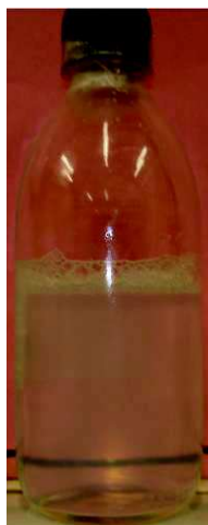
Figure 2.11: Photograph of an obtained PEA nanolatex after filtration and centrifugation. One can see that the dispersion is transparent.
