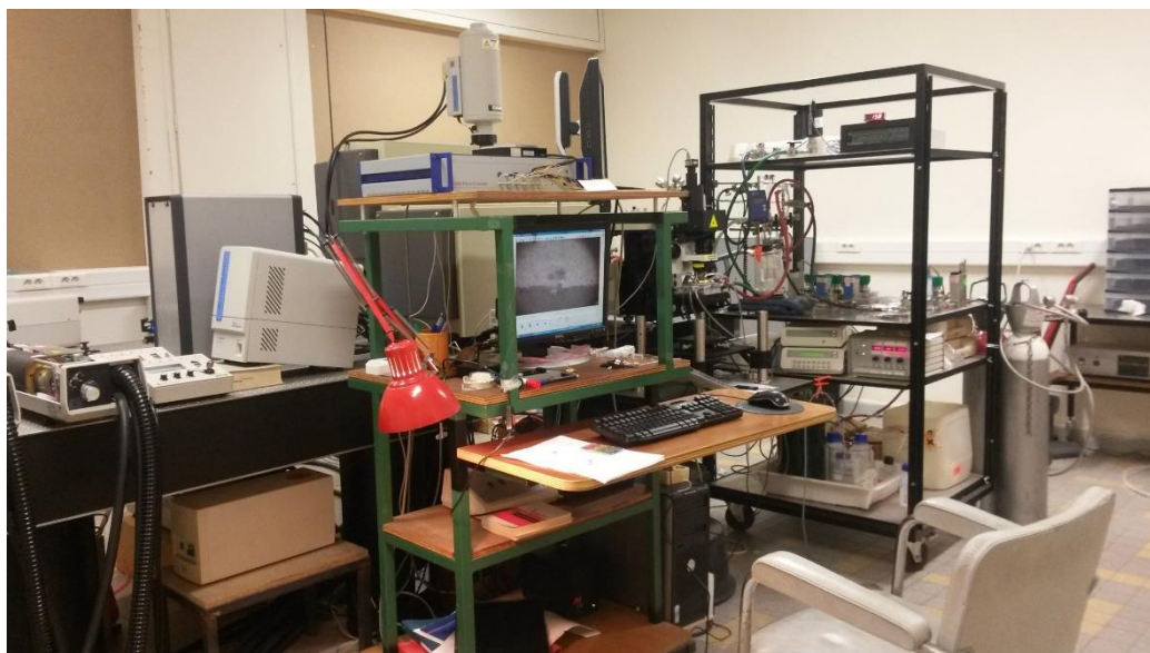
Figure II-1: Raman T64000 with a Linkam cell, equipped with H 2 , O 2 and Ar.
