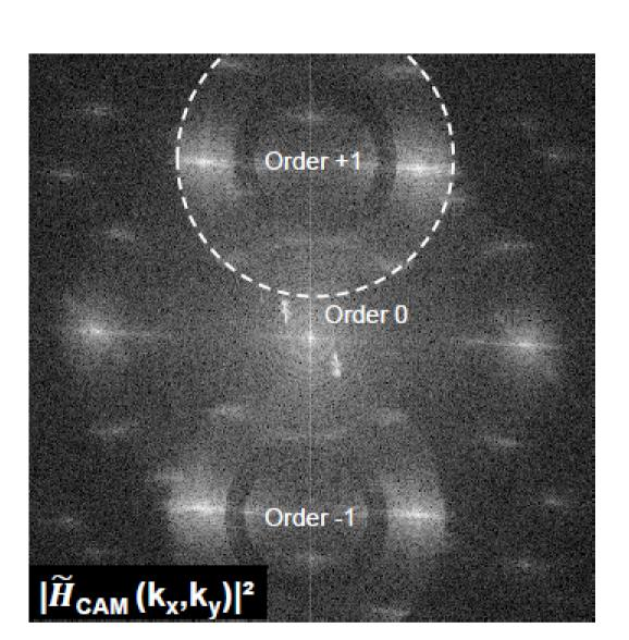
Fourier Transform of the hologram obtained with a 20x/0.5 microscope objective with a phase ring. The double illumination is visible inside the pupil of the MO.
