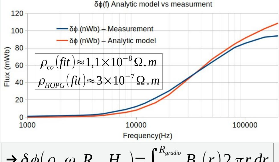
$$\rightarrow \delta \phi(\rho, \omega, R_S, H_S) = \int_0^{R_{gradio}} B_z(r) 2\pi r dr$$
