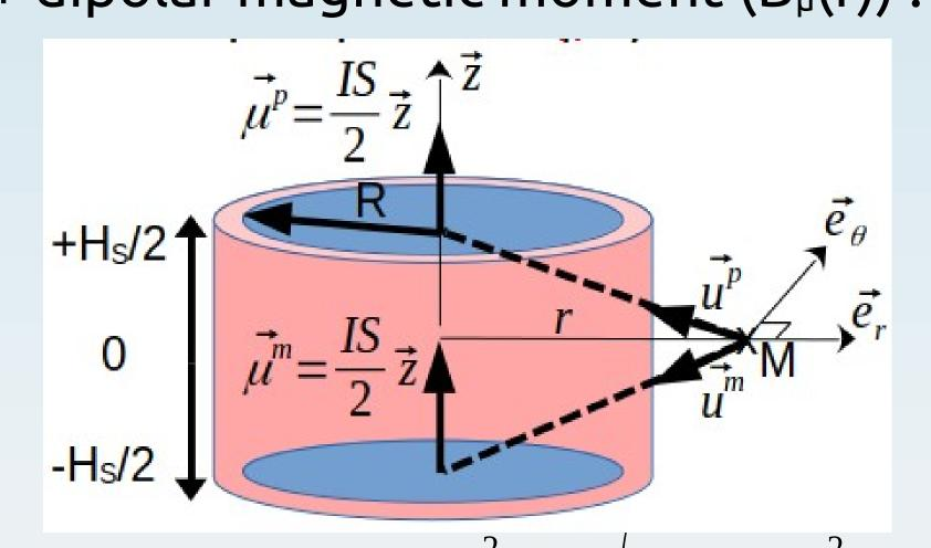
$$B_{z}(r) = B_{sample} + \frac{\mu_{0} I R_{S}^{2}}{4 \left(r^{2} + \left(\frac{H_{S}}{2}\right)^{2}\right)^{3/2}} \left[ \frac{3H_{S}^{2}}{4\sqrt{r^{2} + \left(\frac{H_{S}}{2}\right)^{2}}} - 1 \right]$$
