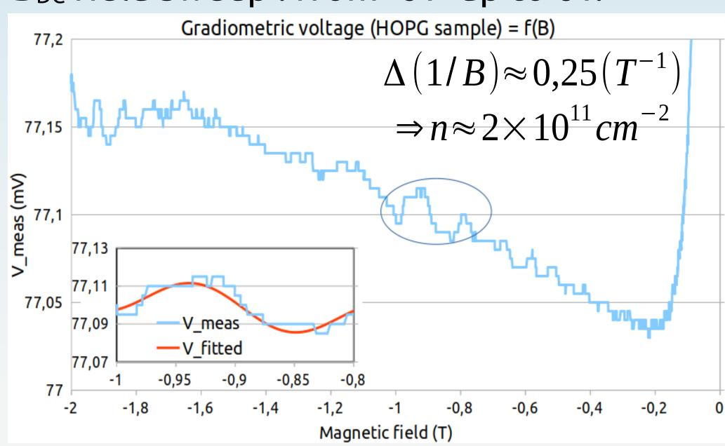
The obtained carrier concentration is consistent with litterature [6]
